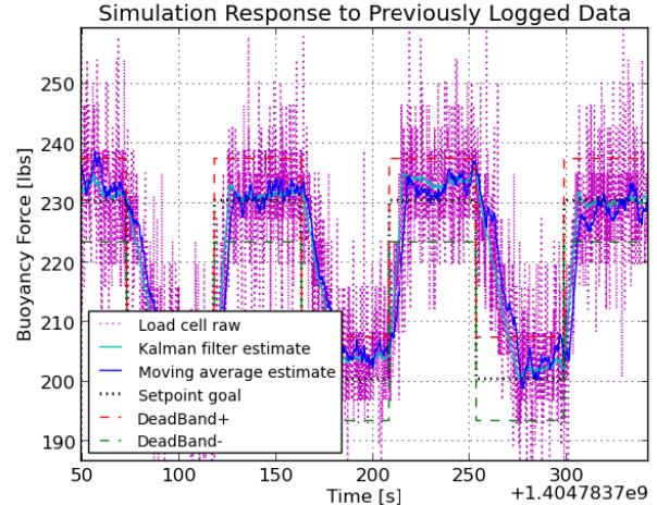
Fig. 7 Moving average filter and Kalman filter response tested in simulation using previously logged data from the AUV load cell
