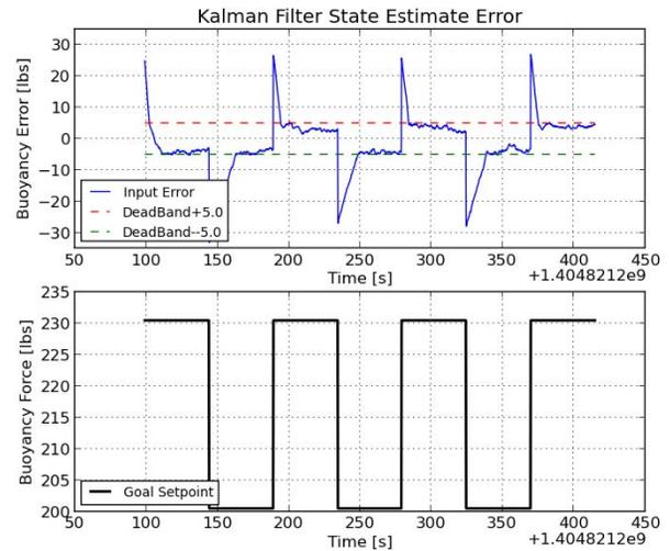
Fig. 11 The Kalman filter estimator responds well to a step input with a deadband of +/- 5 lbs. Once the controlled response reaches a deadband it does not overshoot.
