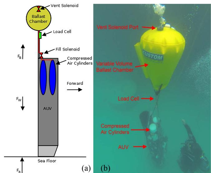
Fig. 1 a) AUV conceptual image in the X-Z plane.  $F_B$  is the buoyant force from the ballast chamber,  $F_W$  is the wet weight of the vehicle, and  $F_R$  is the reaction force between the vehicle and the sea floor. b) Venting of the VBS variable volume ballast chamber during AUV field trials in Hawaii.
