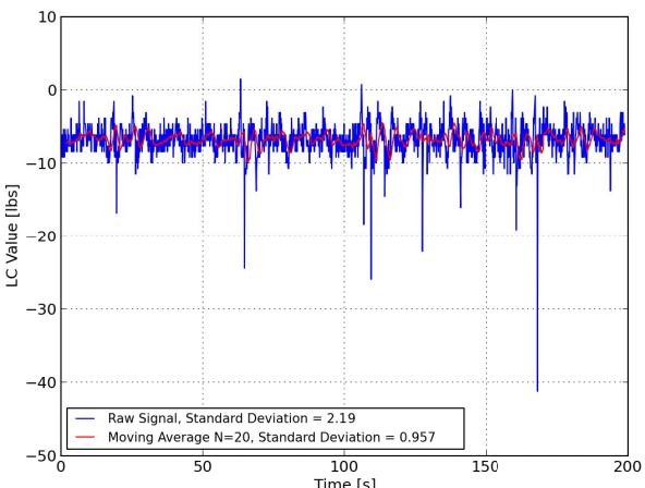
Fig. 2 Raw normal force measurements from the VBS load cell (blue) after passing through a hardware low-pass filter. It is assumed that the remainder of the noise is broadband. The true normal force is constant, but the sensor signal shows a standard deviation of  $\pm 2.19$  lbs due to noise. To meet the system requirements a standard deviation of  $\pm 1$  lb is necessary. The moving average (red) accomplishes this.
