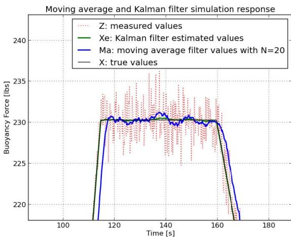
Fig. 6 Close up view of the filter estimates for one step input, taken from (Fig. 5). The time delay on the moving average estimate is easily viewed on the rising and falling slopes of the step response.
