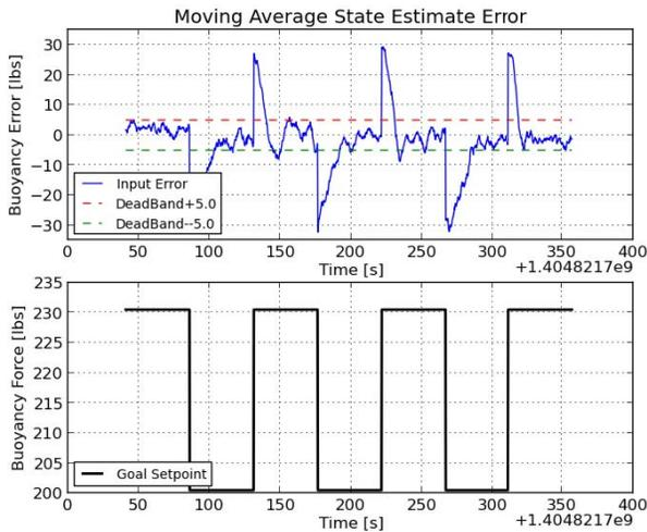
Fig. 9 State estimation error in response to a step input with a bang-bang controller deadband of +/- 5 lbs. This deadband appears to be the operational limit of the moving average filter estimator.
