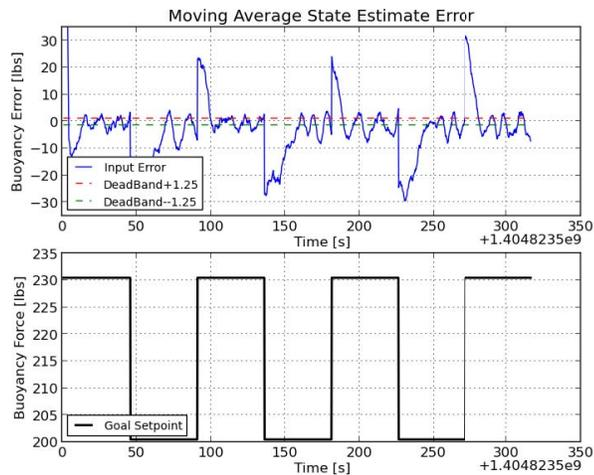
Fig. 10 State estimation error for a deadband of +/- 1.25 lbs. The moving average controller is unstable at this point with the presence of obvious oscillations and continual overshoot beyond the deadband bounds. This would result in rapid cycling of the solenoid valves and likely lead to their failure. Additionally the system is unable to achieve a steady state buoyancy.
