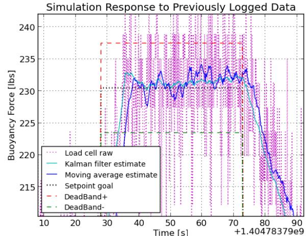
Fig. 8 Close up view of one step input response, taken from (Fig. 7). The Kalman filter estimate (cyan) produces a state estimate ahead of the moving average estimate (blue) and with smaller oscillations about the setpoint value.
