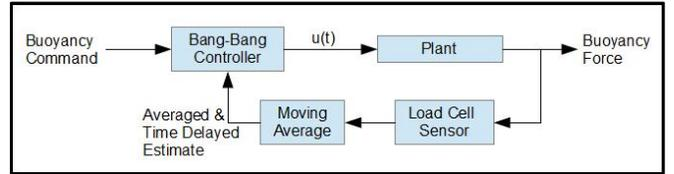
Fig. 3 Moving average bang-bang controller
