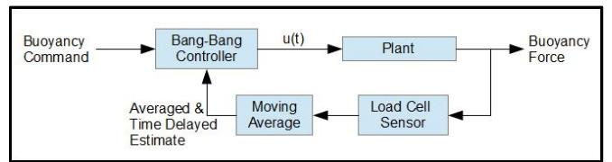
Fig. 3 Moving average bang-bang controller
