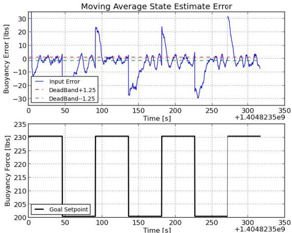
Fig. 10 State estimation error for a deadband of  $\pm 1.25$  lbs. The moving average controller is unstable at this point with the presence of obvious oscillations and continual overshoot beyond the deadband bounds. This would result in rapid cycling of the solenoid valves and likely lead to their failure. Additionally the system is unable to achieve a steady state buoyancy.
