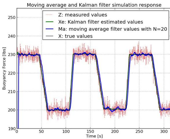
Fig. 5 Moving average filter and Kalman filter tested in simulation. The measured values Z were generated using the true values X and zero mean, additive, Gaussian white noise with a standard deviation of 2.19 lbs. Note the delay in the moving average filter estimates (blue).
