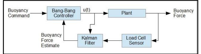
Fig. 4 Model-based Kalman filter bang-bang controller
