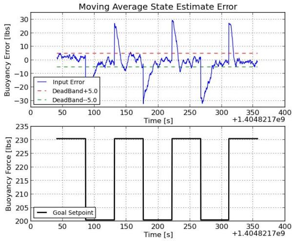
Fig. 9 State estimation error in response to a step input with a bang-bang controller deadband of  $\pm 5$  lbs. This deadband appears to be the operational limit of the moving average filter estimator.
