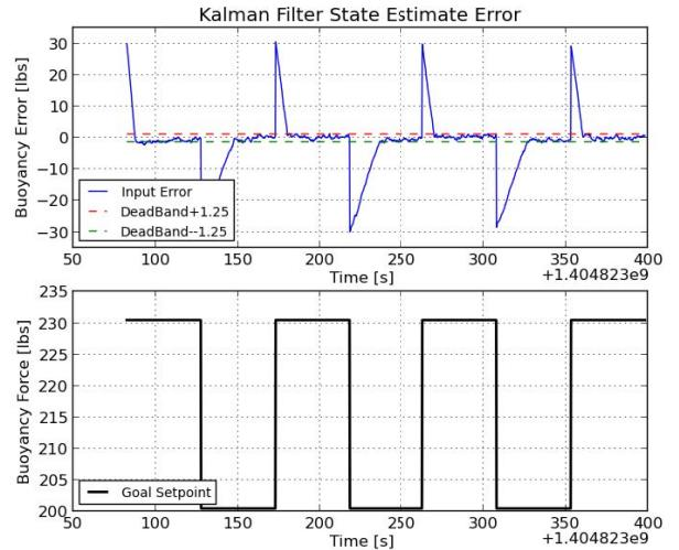
Fig. 12 Kalman filter state estimation response with a control deadband of  $\pm 1.25$  lbs. The filter performs well at this range with no overshoot and quick conversion to a minimal amount of state error. At this range the Kalman filter estimator clearly outperforms the moving average filter.
