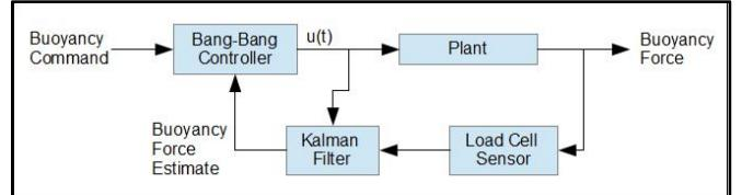
Fig. 4 Model-based Kalman filter bang-bang controller
