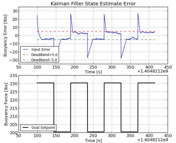
Fig. 11 The Kalman filter estimator responds well to a step input with a deadband of  $\pm 5$  lbs. Once the controlled response reaches a deadband it does not overshoot.
