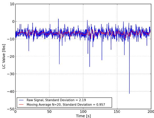
Fig. 2 Raw normal force measurements from the VBS load cell (blue) after passing through a hardware low-pass filter. It is assumed that the remainder of the noise is broadband. The true normal force is constant, but the sensor signal shows a standard deviation of  $\pm 2.19$  lbs due to noise. To meet the system requirements a standard deviation of  $\pm 1$  lb is necessary. The moving average (red) accomplishes this.
