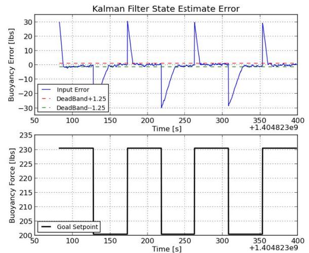
Fig. 12 Kalman filter state estimation response with a control deadband of +/- 1.25 lbs. The filter performs well at this range with no overshoot and quick conversion to a minimal amount of state error. At this range the Kalman filter estimator clearly outperforms the moving average filter.
