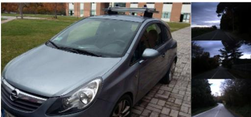
Fig. 7: Car setup used for collecting the Perugia Countryside Dataset. On the right, some sample images of the recorded sequences are shown.
